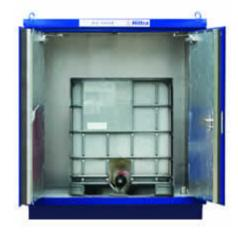
Article number 210170250 Fire resistance F60 according to NEN6069 (Efectis report) Dimensions uitw. WxDxH 2090 x 1830 x 2590 mm Dimensions int. WxDxH 1810 x 1470 x 1925 mm Storage capacity 1x IBC, 1x chemical or 1x europallet Load capacity of slatted 1250 kg/m2 floor Steel lacquered with Collection box galvanized grid floor
