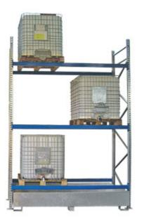
Article number 18536 Suitable for 6x IBC, 24x 200L drum, 6x chemical pallet or 9x euro pallet External dimensions approx. 2930 x 1100 x 4000 WxDxH mm Box width approx. 2700 mm Drip tray BxDxH approx. 2650 x 1300 x 493 mm Contents collection box approx. 1100 kg Underride height approx. 100 mm Weight rack / bin approx. 196 kg / approx. 107 kg
