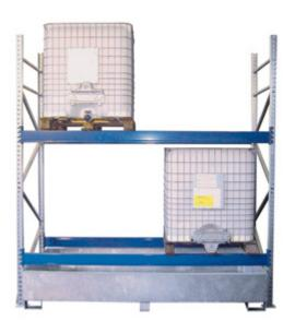
Size Hiltra drum rack type 4 Article number 18535 Suitable for 4x IBC, 16x 200L drum, 4x chemical pallet or 6x euro pallet External dimensions approx. 2930 x 1100 x 3550 WxDxH mm Box width approx. 2700 mm Drip tray BxDxH approx. 2650 x 1300 x 493 mm Contents collection box approx. 1100 litres Underride height of drip approx. 100 mm tray Weight rack / bin approx. 153 kg / approx. 107 kg
