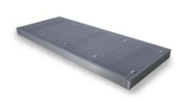
Size Coupling floor element model FW 5  $\sim$  (2.5 m2) Article number 8301 Dimensions LxWxH external 2500 x 1000 x 118 mm Collection capacity 210 liters Weight approx. 138 kg Floor load 6500 kg/m<sup>2</sup> Field pressure load 600 kg (20x20 cm) Material made of galvanized steel 3 mm S235JR
