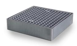
Size Coupling floor element model FW  $1\sim (0.25 \text{ m2})$ Article number 8320 500 x 500 x 118 mm Dimensions LxWxH external Collection capacity 20 liters Weight approx. 20 kg Floor load 6500 kg/m<sup>2</sup> Field pressure load 600 kg (20x20 cm) Material made of galvanized steel 3 mm S235JR
