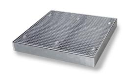
Size Coupling floor element model FW 3 ~ (1 m2) Article number 8303 Dimensions LxWxH external 1000 x 1000 x 118 mm Collection capacity 83 liters Weight approx. 66 kg Floor load 6500 kg/m<sup>2</sup> Field pressure load 600 kg (20x20 cm) Material made of galvanized steel 3 mm S235JR
