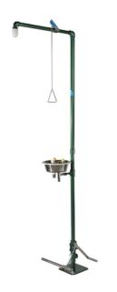
Size Emergency and eye shower MBS300-30 (stainless steel) Article number 99999979 Material Eyebath stainless steel, pipes steel Pipework **RVS** Shower Stainless steel pull rod, Operation eyebath Stainless steel push bar Water flow Shower 80 ltr/min, eyebath 12 Itr/min Above ground, 1¼" BSP internal Water supply thread Implementation Self-draining for indoor use
