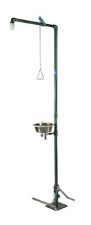
Size Emergency and eye shower MB300-30 Article number 99999979 Material Eyebath stainless steel, pipes steel Pipework Galvanized ShowerRVS pull rod, stainless Operation steel eyebath, push bar Water flow Shower 80 ltr/min, eyebath 12 Itr/min Above ground, 1¼" BSP internal Water supply thread
