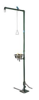
Size Emergency and eye shower MBS300-30 (stainless steel) Article number 99999979 Material Eyebath stainless steel, pipes steel Pipework **RVS** Shower Stainless steel pull rod, Operation eyebath Stainless steel push bar Water flow Shower 80 ltr/min, eyebath 12 Itr/min Above ground, 1¼" BSP internal Water supply thread Implementation Self-draining for indoor use
