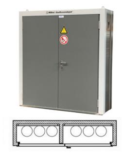
Size Hiltra F60 gas bottle facade cabinet model GK-MS 6-bw Article number 161800200 CAUTION !!! Overhang above the door has been removed Dimensions external 2515 x 630 x 2330 mm **WxDxH** Dimensions internal BxDxH 950/1125 x 360 x 2100 mm Door leaf size WxH 2070 x 2050 mm 6x 50 liter standard cylinder Capacity Weight approx. 760 kg
