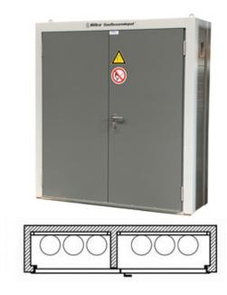
Size Hiltra F60 gas bottle facade cabinet model GK-MS 6 Article number 160800200 CAUTION !!! Overhang above the door has been removed Dimensions external 2265 x 630 x 2330 mm **WxDxH** Dimensions internal BxDxH 1985 x 360 x 2100 mm Door leaf size WxH 1820 x 2050 mm 6x 50 liter standard cylinder Capacity Weight approx. 665 kg
